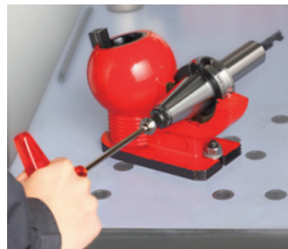
Clamping DETa-1 Collet( DTB )
