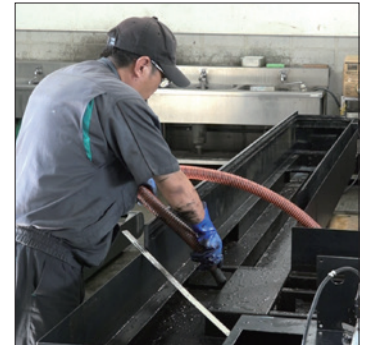
Periodic cleaning of the coolant tank
