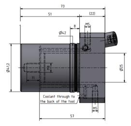
\*\*On this design, you can choose to port coolant through the M5 hole in the bottom or top of the holder.
