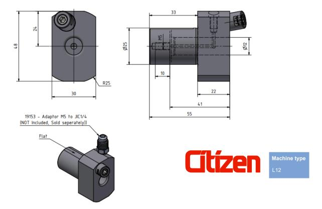
This L12 holder will also fit into an existing Tsugami holder 3282-Y211 Uses R1912.xxxxx reduction sleeves, E7321.12000, 19153, S041
