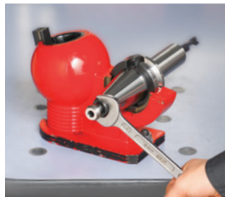
Retention knob tightening
