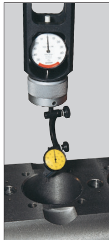
Usage example for test indicator
