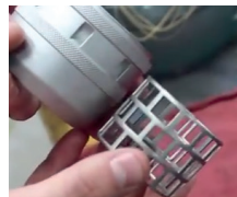
Machining of cavity using throchoidal milling with ETP HYDRO-GRIP HD
